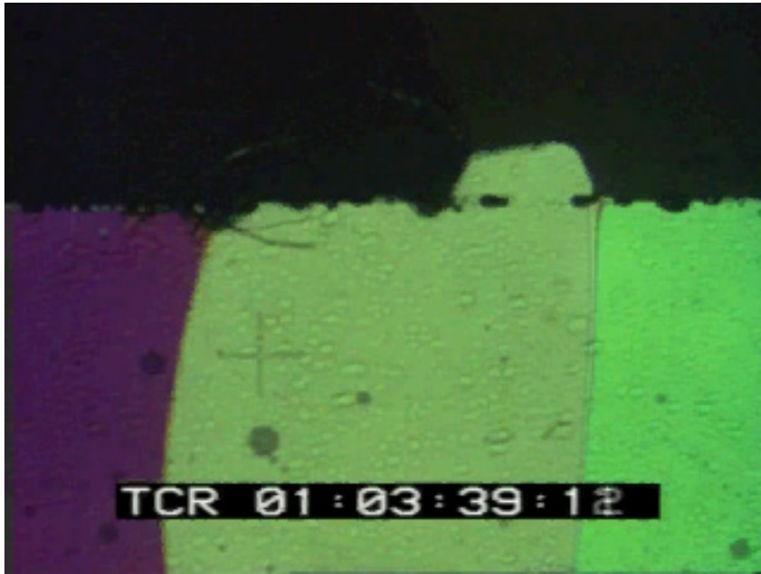
Movie 3 - A pure shear deformation of four ice grains over \approx 2.5 days.
