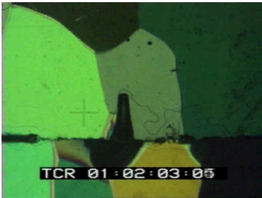
Movie 1 - Pure shear deformation in polycrystalline ice over \approx 2.5 days.
