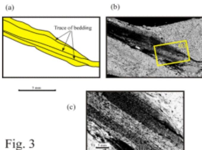
**Fig 3** Bedded shale clast. (a) is a tracing of (b) which is a general view showing bedding-parallel to the long dimension of the clast. Clast is shown in yellow. (c) is an enlargement of the area indicated in (b) and shows the parallelism of the mica foliation and bedding. Photographs with crossed polarisers.
