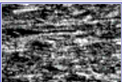
[BHQ deformed by a combination of sinistral simple shear \( \$\gamma = 2.1\$ \) and shortening \(~50%\) at 800°C, 10-5/sec and 1200 MPa; regime 2 dislocation creep.](#)
