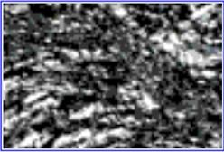
**TA shortened 35% at 900°C, 10<sup>-6</sup>/sec, and 1200 MPa; narrow zones of very fine recrystallized grains (regime 1 dislocation creep) allow localized dextral shear.**
