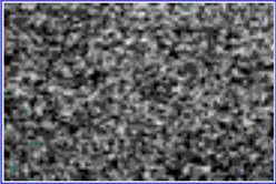
**Arkansas novaculite (original  $d = 5 \mu\text{m}$ ) shortened 54% at  $900^\circ\text{C}$ , 10-6/sec and 1200 MPa ('wet'); transition between regime 2 - 3 dislocation creep.**
