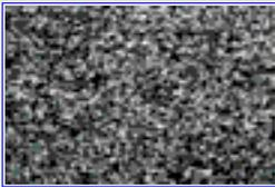
[Arkansas novaculite \(original d = 5 μm\) shortened 54% at 900°C, 10-6/sec and 1200 MPa \('wet'\); transition between regime 2 - 3 dislocation creep.](#)
