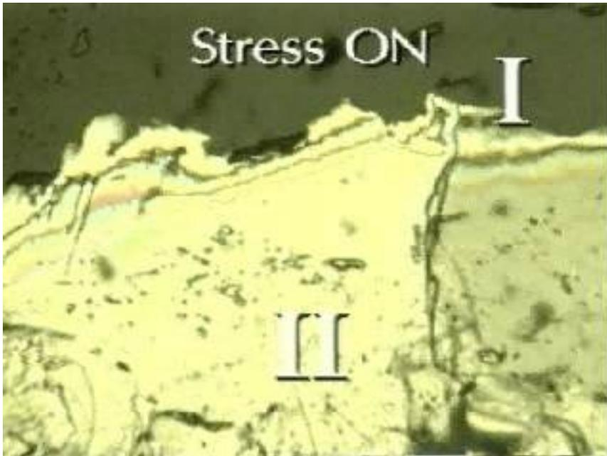
**Fig. 12** This static image shows another example of transformation from I to II under stress (actually taken from the earlier movie). Stress caused the phase boundary to move northwards- phase I was consumed. The movie here shows a final example of I - II transformation under stress where the phase boundary is particularly unstable although it is not known why. No stress initially but the boundary begins to move erratically as soon as stress is applied. Shortening is E-W.
