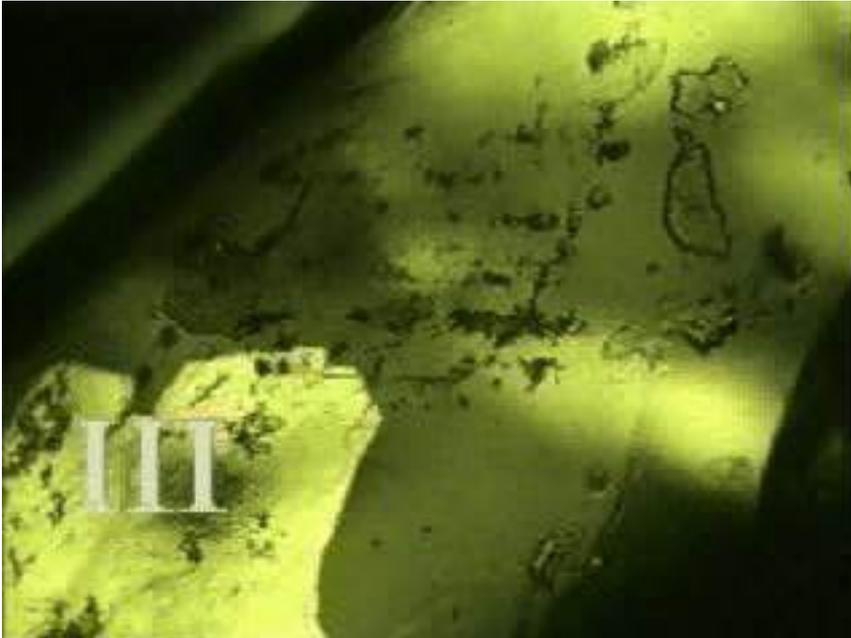
**Fig. 4** Single crystal of Phase IV transforms on heating at about  $32^\circ\text{C}$  into phase III. A 'faceted' interface advances slowly but steadily from the bottom left corner.
