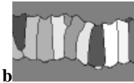
Figure B4. Movies showing the effect of fracture width on the vein texture for the prismatic "mineral". All parameters are kept the same, except the vertical opening distance, which is (a) 2 pixels, (b) 4 pixels and (c) 16 pixels. See text for discussion.
