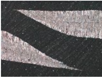
Figure 17. Tips of two parallel en échelon antitaxial fibrous calcite veins. Mean fibre width increases slightly from the median line outwards, which indicates that growth was outwards (antitaxial). Fibre shape is symmetric around the median line, except near the tips. Growth and propagation of the veins caused bending of the shale "bridge" in between. Tapley Hill Formation, Opaminda Creek, Arkaroola, South Australia. Width of view 13 mm, crossed polars.
