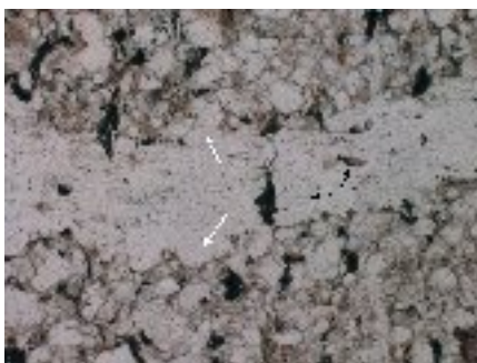
Figure 13. Photomicrograph of stretched quartz crystals in a sandstone hosted vein in (a) plane polarised light and (b) cross polarised light. The vein material was formed by adding material to existing grains in the sandstone. White arrows indicate parts of a stretched vein crystal that formed two halves of one grain before the vein formed. Vein wall parallel dust trails and wall rock inclusions (black arrows) indicate that this vein formed by repeated crack-sealing, which can also
