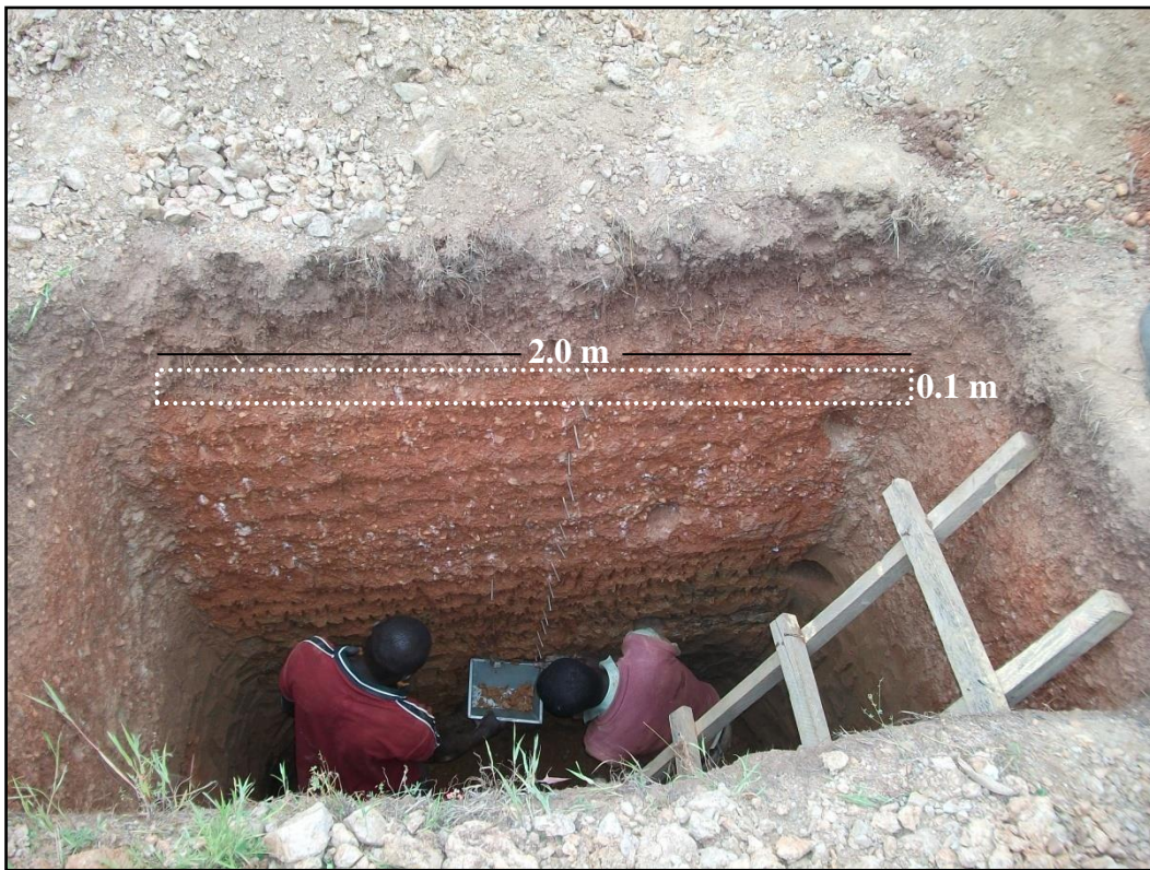
Fig. 4.18 A typical vertical panel sample collection at 10 cm intervals of a well-lithified regolith profile. Sample spacing is marked by the nails and white rectangle shows panel sampling dimensions.
