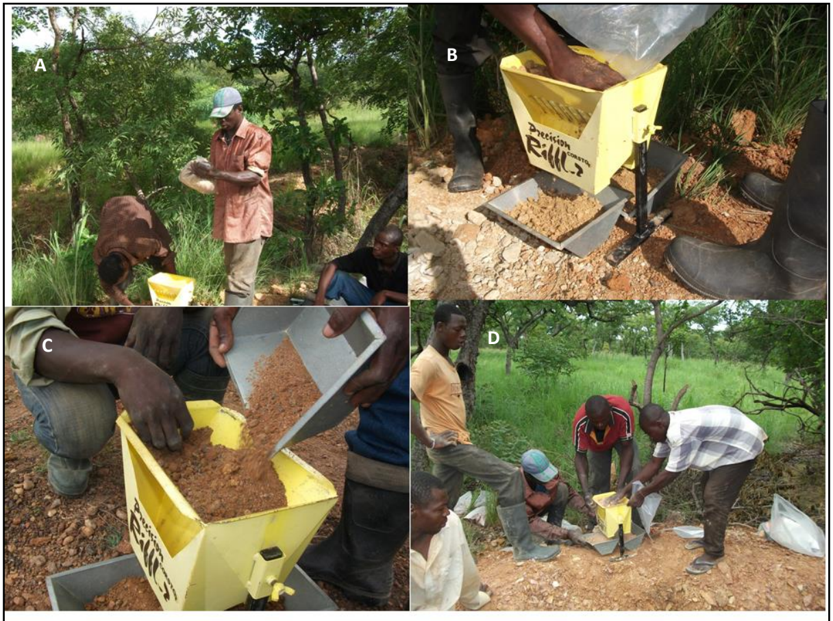
Fig. 4.20 Sample splitting stages in the field: a). manual sample homogenization in plastic bag, b) clump disaggregation and oversize removal, c) sample splitting, and, d) library and laboratory samples bagging.
