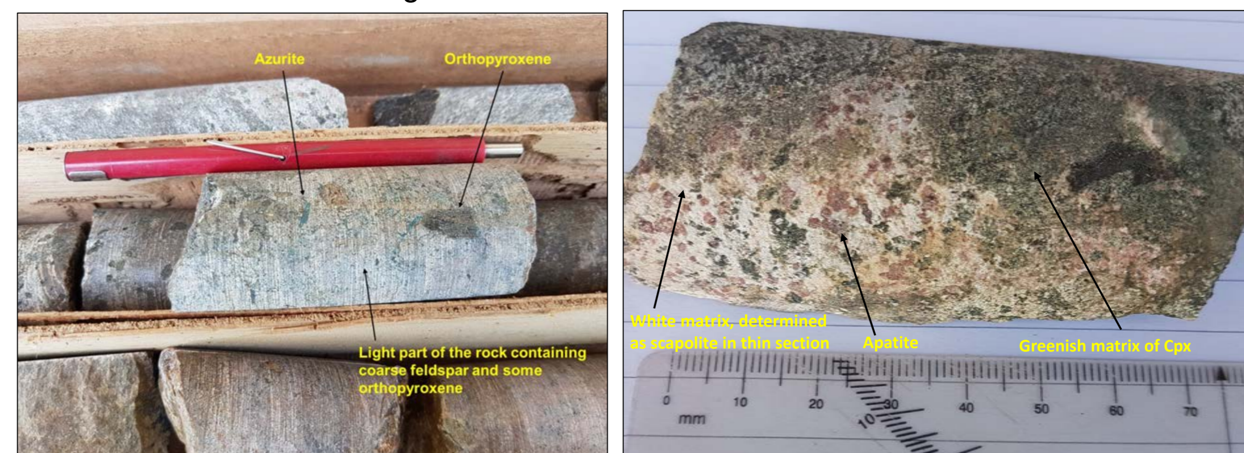
Figure 5: Leucosome of migmatitic granulite containing copper minerals (left); Ca-silicate granulite showing high concentration of apatite (right)
