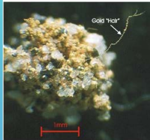
Mass of delicate gold crystals intergrown with both angular and rounded sand grains. Note extremely delicate gold "hair" extending from mass.
