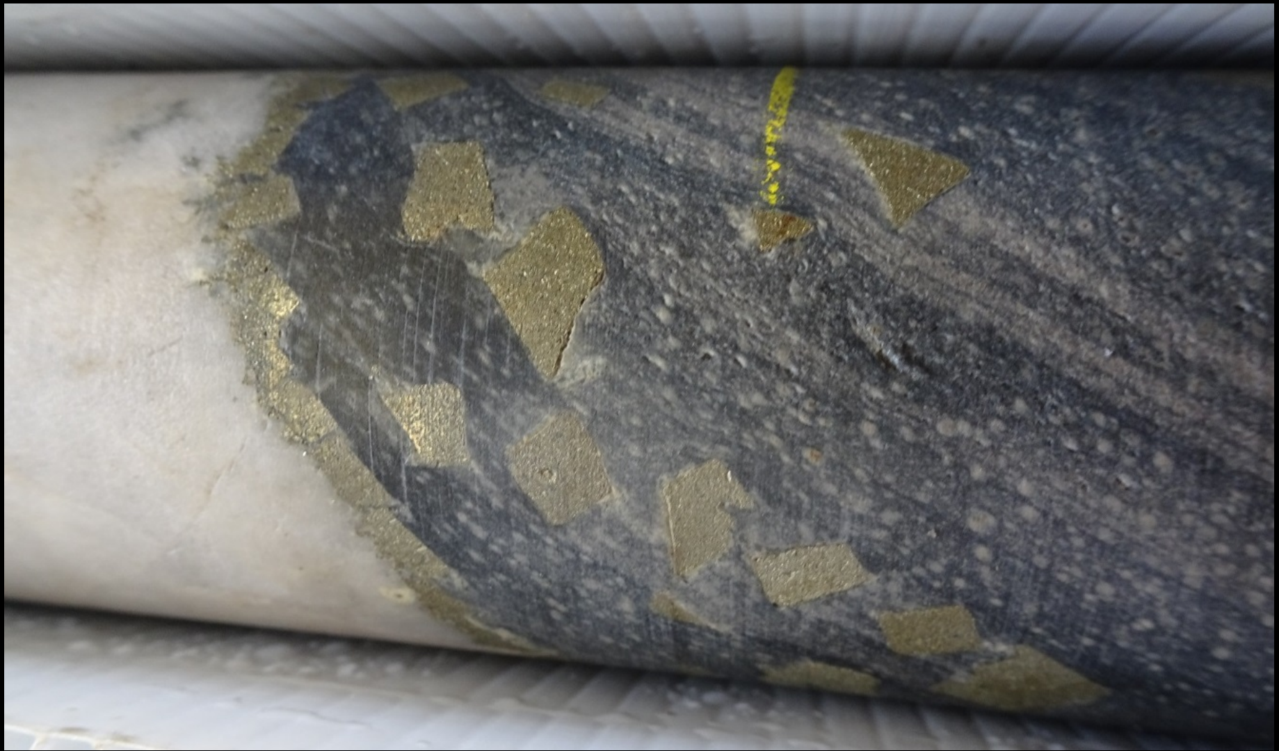
Gold-bearing pyrite in metagreywackes and quartz vein IAMGOLD Rosebel Gold Mines
