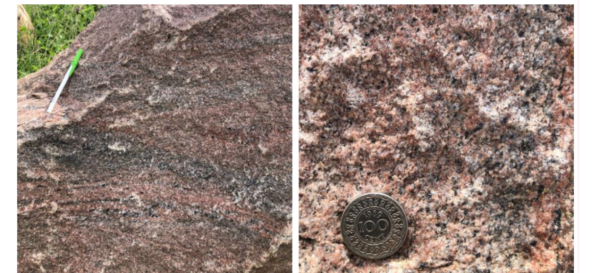
Figure 12: Photographs of the pink Tibiti granite. The left photograph shows a weak banded texture in the rock and the right photograph, the medium to coarse grained texture is presented.
