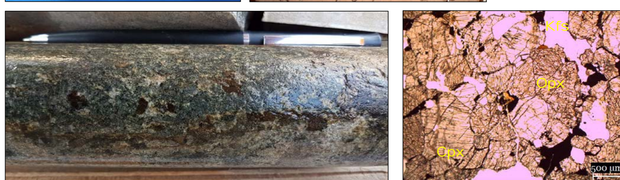
Figure 4: Ca-silicate granulite with cpx and opx (left); Thin section in PPL showing cpx, opx, K-feldspar and opaque minerals between contacts (right)
