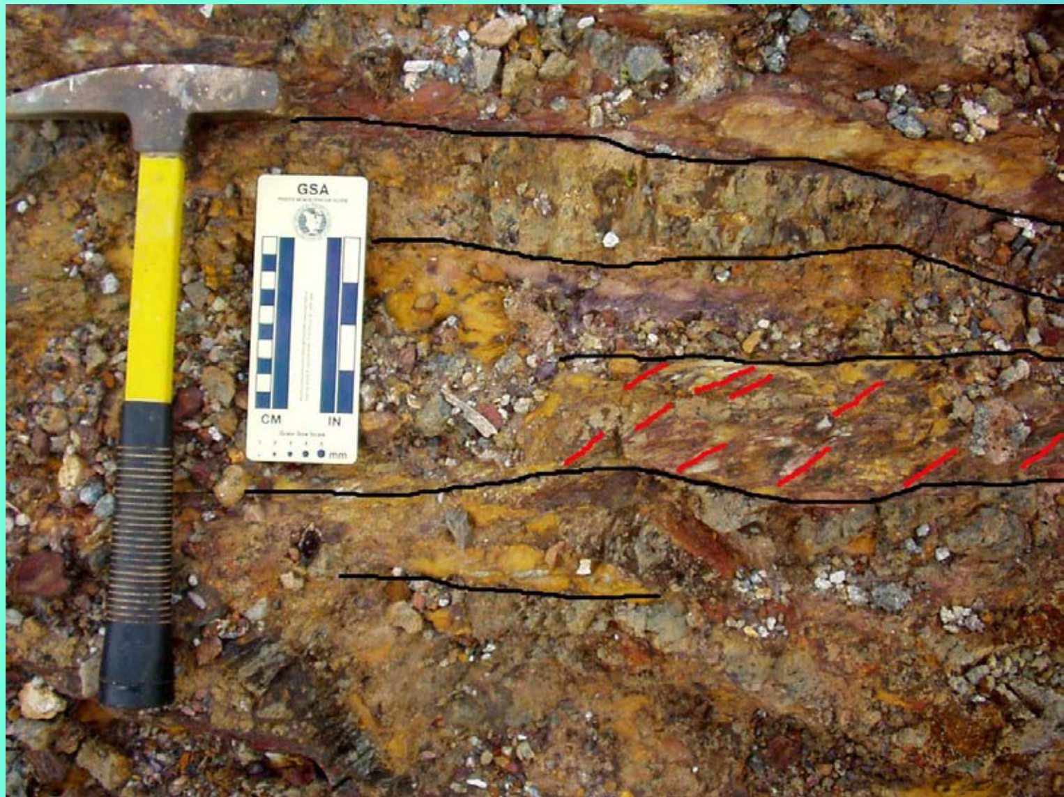
Well developed c-s fabric indicating dextral shear, center of Gowtu Bergi pit, Merian 2 Area, Nassau Au Project
