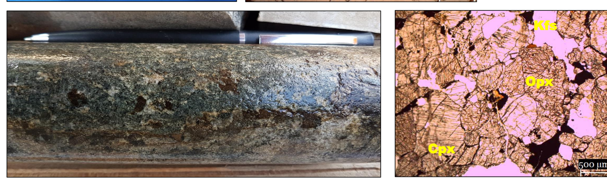
Figure 4: Ca-silicate granulite with cpx and opx (left); Thin section in PPL showing cpx, opx, K-feldspar and opaque minerals between contacts (right)
