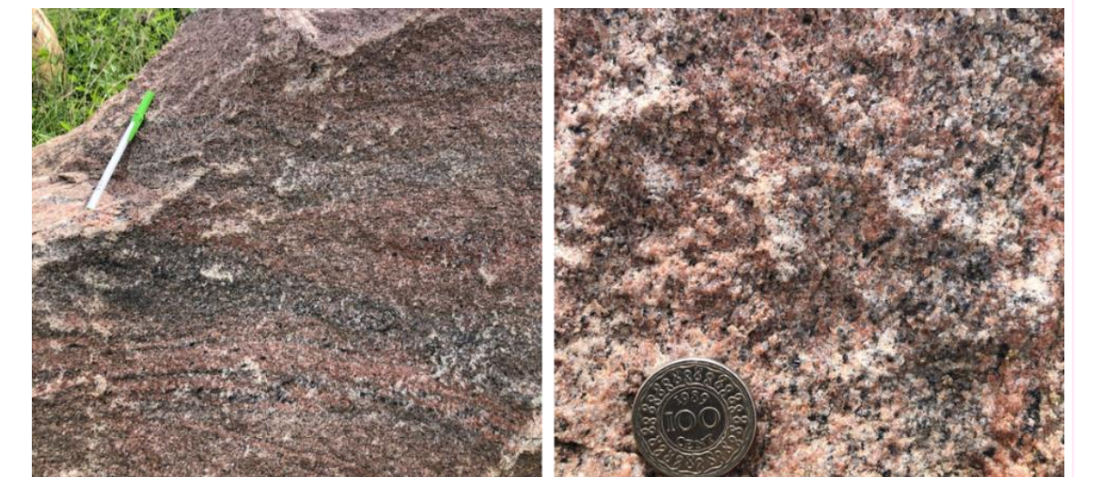
Figure 12: Photographs of the pink Tibiti granite. The left photograph shows a weak banded texture in the rock and the right photograph, the medium to coarse grained texture is presented.
