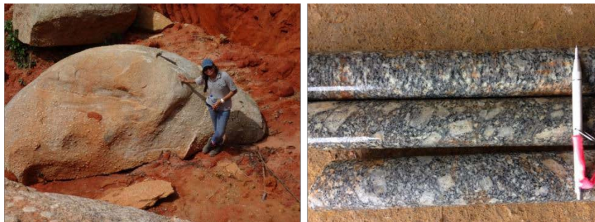
Figure 2: The left image shows the size of the boulders of the Akinto Soela Granite in an exploration pit. The image on the right illustrates drill core samples of the Akinto Soela granite, clearly showing the well-defined K-megacrysts in a coarse-grained texture.
